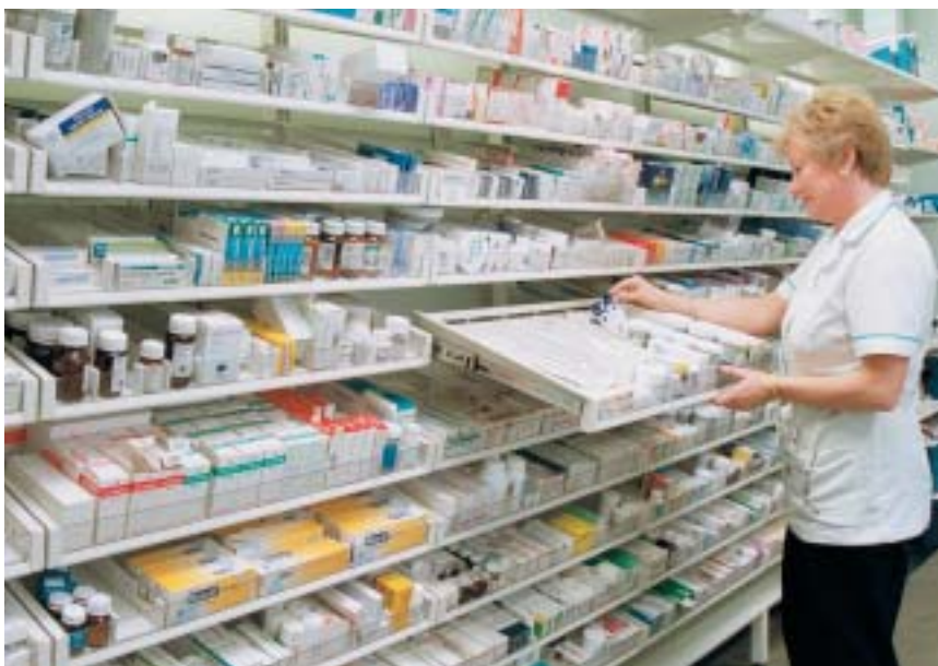
Sloping trays withdrawn for convenient replenishment. Hospital pharmacy, United Kingdom.
