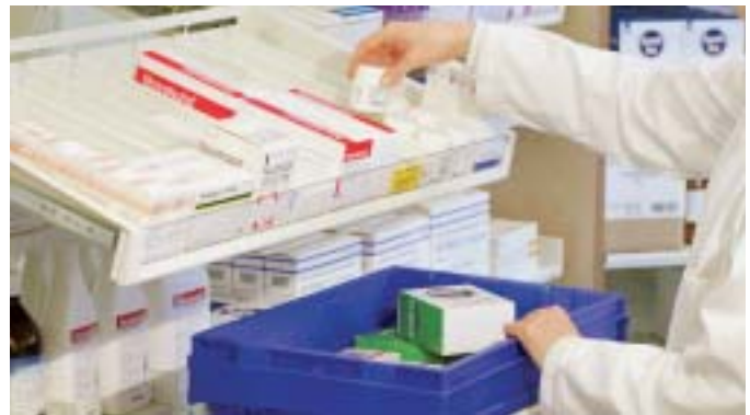
The Combi trays can be drawn out for quick refilling at the back to give “First-in first-out” stock rotation.
